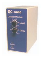
C-mac<sup>®</sup> current monitoring relay, type RC30, and voltage monitoring relay, type RV30 are universal metering relays, each supplied with 3 metering ranges, automatic detection of AC or DC input signal, plus a 24 VDC output voltage, for the supply of external sensors or the like.
