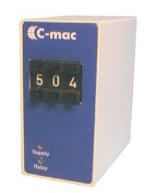
C-mac<sup>®</sup> module type RD53 is a digital pulse counter module, selectable as pulse divider or preselection relay. The pulse inputs can be activated from a mechanical contact, a transistor or a NAMUR sensor, and the reset input can be activated from a mechanical contact or a transistor. The unit is supplied with a "slave" transistor output, in this way several units can be connected to the same pulse sensor.
