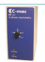
The C-mac<sup>®</sup> module type RP31 meters its own 3-phase supply voltage, and if the phase sequence is correct and the phase asymmetry is below the adjusted level, the output relay is activated.
