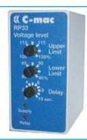
The C-mac<sup>®</sup> module type RP33 meters its own 3-phase supply voltage, and checks that all 3 phase-neutral voltages are within the adjusted limits, and in that case, the output relay is activated.
